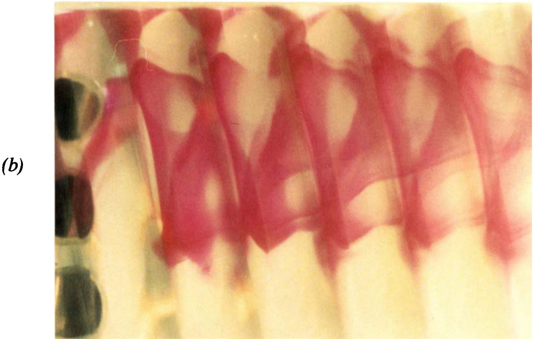
FIGURE 1. (a) Flow between two 45° plates. Dye is produced at a circular electrode ( Re=70 ). (b) Flow between two 80° plates. Dye is produced at a circular electrode ( Re=80 ).
